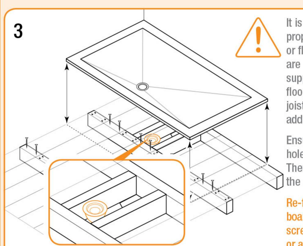
It is essential that the floor boards are properly secured, ensuring no movement or flex. Any joins in the floor boards that are not supported by a joist must be supported by separate noggin(s). Any floor boards that show flexing between joists MUST also be supported by additional noggin(s).
