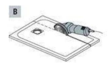
the installer must mark the cutting line with a pencil (A) and then with a tile cutter, cut off the excess (B)
