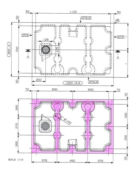
Compared to the competitors, the shower tray is lighter because the bottom is "emptied", except for the fixed-pitch ribs which are used to unload the weight on the ground, here in violet.
