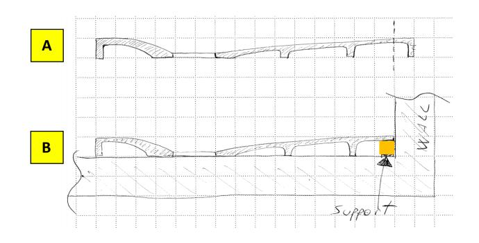
In the case of installation of cut shower trays (A), the installer must put a support/thickness so that the weight can be unload to the floor (B).
