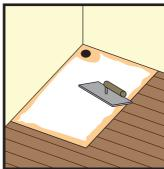
**Step 5)** Run a large bead of silicone on all edges that will contact the walls. Bed the tray with fitted waste into the sand and cement mix making sure the tray is 100% level on all sides. Repeat water test 2.
