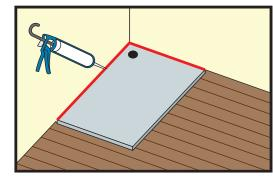
**Step 6)** Run a further bead of neutral mould resistant silicone around the rims of the tray Adjacent to all walls. Allow all aspects of material to cure according to the instructions.
