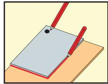
**Step 2)** using a sheet of marine plywood with a minimum thickness of 12mm mark the trays perimeter and waste hole. Fit all waste services before securing your plywood to your joists. (For sizing please refer to **Fig A** on opposite page)
