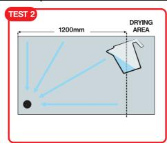
End waste trays greater than 1200mm incorporate a drying area at the non waste end, this area is nominally flat and should not be incorporated in the water test area. Centre waste trays drain test both ends.
